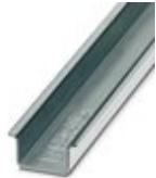
DIN rail, unperforated, Standard profile, width: 35 mm, height: 15 mm, similar to EN 60715, material: Steel, Galvanized, white passivated, length: 2000 mm, color: silver
